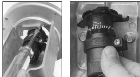
Removing the adjuster from the front
